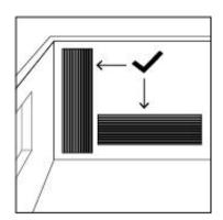
The panels can be installed vertically or horizontally as desired.
