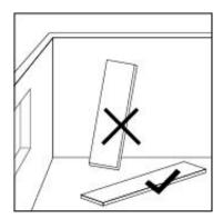
To prevent warping, never store packages and panels upright; instead, lay them flat on a level surface. Protect the panels from moisture. Expansion and contraction occur under changing humidity conditions. Moisture promotes mold growth..
