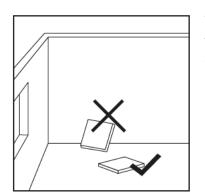
To prevent warping, never store packages and panels upright; instead, lay them flat on a level surface. Protect the panels from moisture. Expansion and contraction occur under changing humidity conditions. Moisture promotes mold growth.
