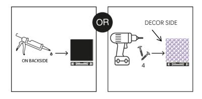
The wall panels can either be screwed or glued to the wall.
