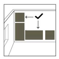
The panels can be mounted vertically or horizontally as desired.
