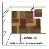
The graphic below shows where the connector strip can be used if the following arrangement of the panels is be choosen.
