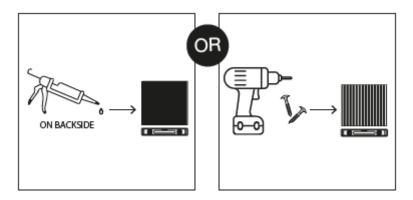
The acoustic panels can either be screwed or glued to the wall.
